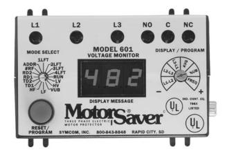
**Model 601** Three Phase Voltage Monitor is a fully programmable electronic voltage monitor designed to monitor three phase systems. It can be used as a stand alone product or the communication port can be used to form a network and monitor the motors from a laptop or desktop computer; or other control system.
